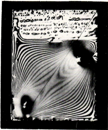
Figure 8. Oil on pallet stone after several months' operation.
