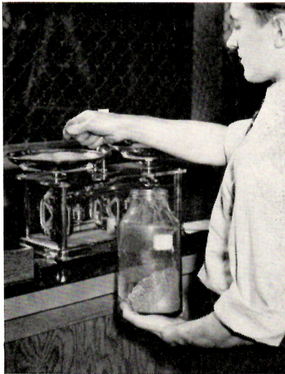
1. Each metal employed in the alloy for Elinvar Extra is weighed on laboratory type scales.
