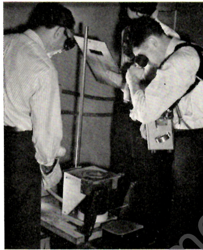
2. Metallurgists frequently check temperatures against processing time in making a "heat" of Elinvar Extra.
